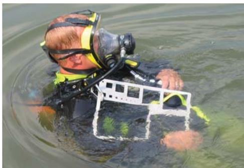
DNR technician Mike Everhart wearing an audio diving mask, uses a gravelometer to measure the size of rocks in the streambed then relays information to surface.
